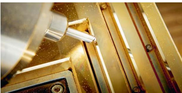
RIGHT: A line that will become a diamond cut in the finished appearance is milled up to five times.
